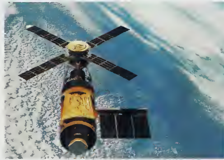
U.S. Skylab in Earth orbit, photographed February 8, 1974, by the final astronaut crew from the Skylab 4 Command Module. The makeshift sun shield and underlying "parasol" on the main part of the space station were installed by the first two crews to cover damage done to Skylab's protective shielding during launch.
